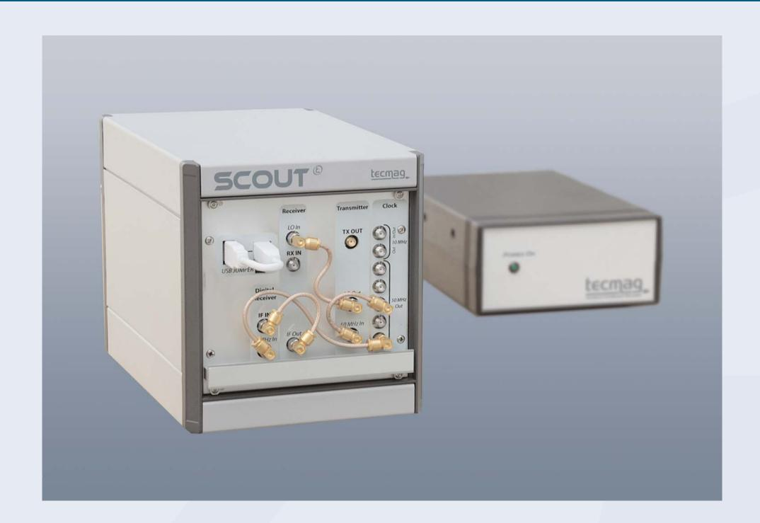
Scout<sup>™</sup> is a compact, expandable, cluster-based spectrometer. The single master cluster measures 6.5" x 7" x 10" with an external power supply. The master cluster contains one broadband transmitter and one digital receiver that can be connected to a Windows 7 Pro 64-bit computer, via an USB 2.0 interface. The optional slave cluster allows expansion with a second identical DC to 300 MHz transmitter or gradient control for imaging or diffusion experiments.
